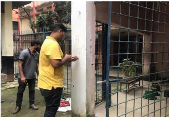
Re-bounce hammer test
