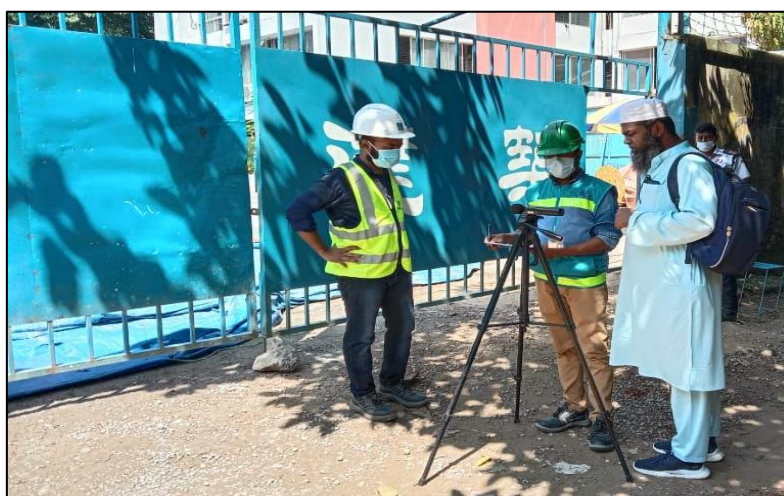
The noise level is assessed using a decibel meter by a third-party laboratory at URU construction site
