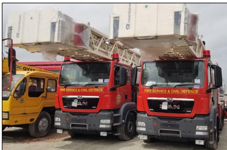
Turn Table Ladder (64 m) for FSCD
